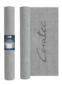
Water-impermeable, seals cracks, double-sided fleece-coated polyethylene sealing membrane. For secure, flexible sealing and decoupling in interior areas, showers and bathrooms before tiling work in accordance with DIN 18534 Part 5 in water exposure classes W0-I "low", W1-I "moderate" and W2-I "high".
